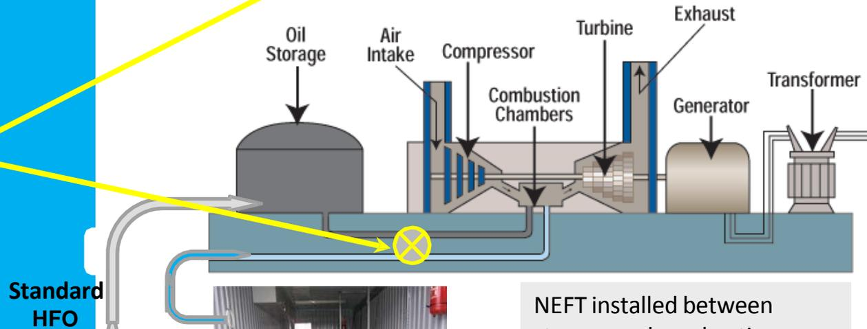
NEFT installed between storage and combustion. Processed HFO into Nano-Emulsion Fuel injected immediately
