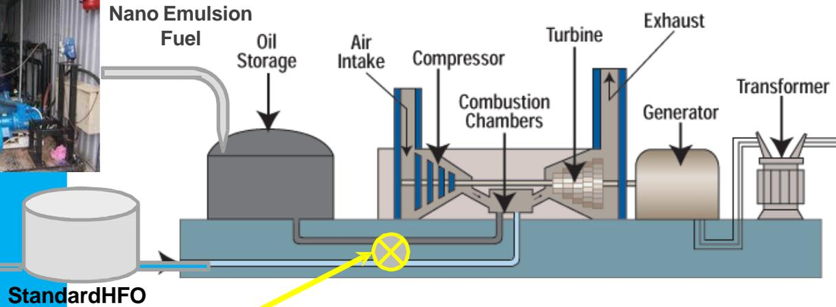
Control valve allows user switch back to standard HFO in case of need and to avoid disruption to energy production
